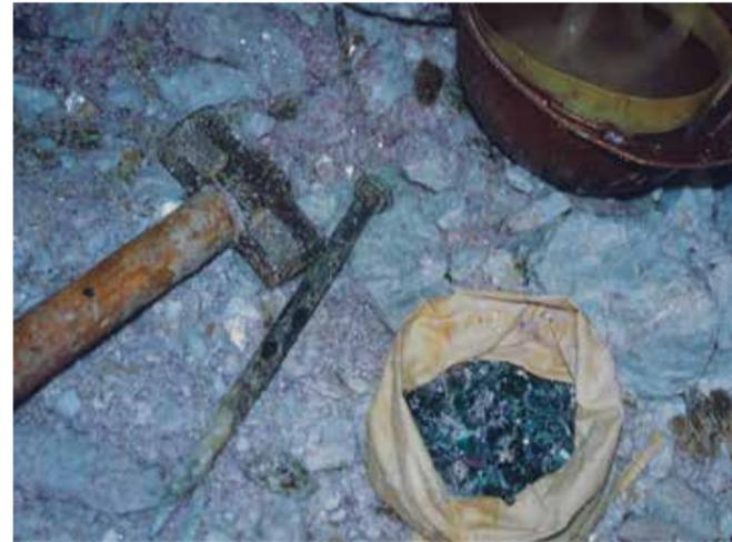
Tools used in the mining process and a bag of the gems recovered.
