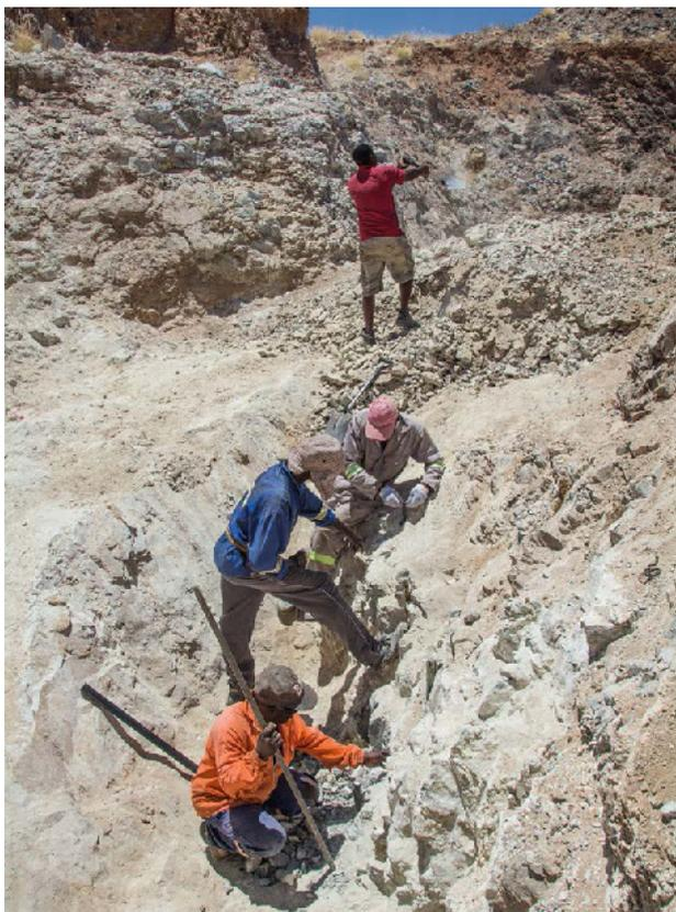
**Figure 7:** Demantoid is mined from a hard layer of calc-silicate rock at the Parrot mine using hand tools. Photo by B. M. Laurs.
